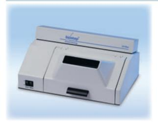
The UV-Box combines two UV-tubes for 254 and 366 nm in one unit and allows inspecting thin-layer chromatograms in an undarkened room.
