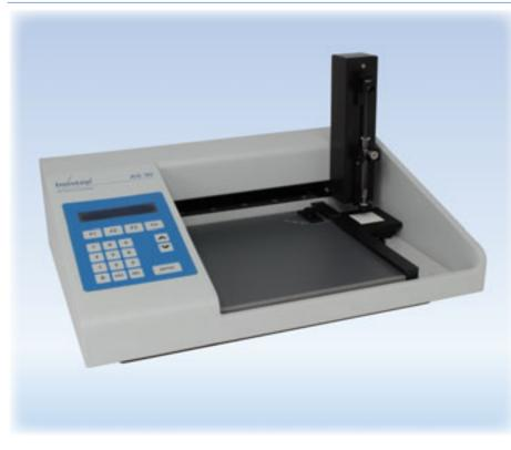
The HPTLC-Applicator AS 30 is a decisive contribution towards modern GxP-conform thin-layer chromatography and works according to the spray-on-technique. A stream of gas carries the sample from the cannula tip onto the HPTLC plate - therefore, compressed air is needed.
