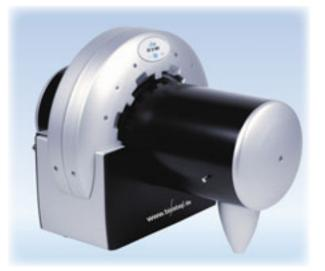
Today radiography is not done anymore by X-ray film but uses modern technology of phosphor image plates in combination with laser excitation and latest photomultiplier tube technology to generate a digital image with much higher dynamic range. Second, unlike film, a phosphor image plate can be reused: plates can be "erased" by exposing the plate to red light. For more information in general and detail see special flyer!
