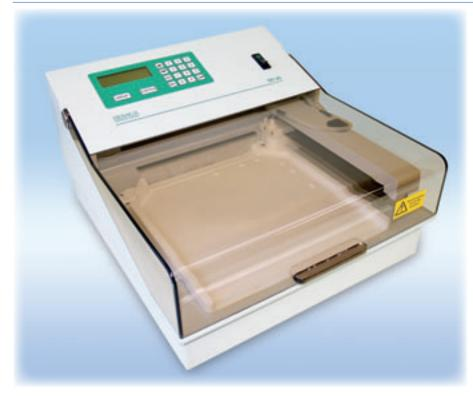
The ChromaJet DS 20 presents a completely new derivatization concept. Reagents are sprayed on thin-layer plates or foils with the highest precision under microprocessor or computer control. The distinction from manual spraying lies in the great reduction in the quantity of reagent required, the almost complete absence of aerosol formation and the evenness of the spray pattern.
