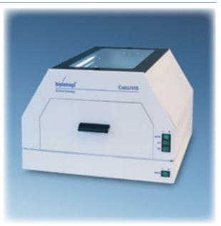
each other. The observation plate of polyacrylate glass provides adequate protection from reflecting short-wavelength UV light. However, the protective goggles included with each unit should be worn for your own safety. For transmission light illumination, the CabUVIS has a special white light 8 Watt tube that is built-in the base. It is covered by a matted polyacrylate glass plate and allows the uniform illumination of objects up to 200 x 200 mm in size.
